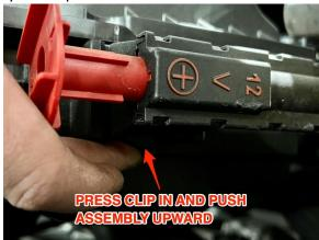
2.4. Remove the airbox by pulling up on the front to pop it out of the rubber grommets, popping the air intake hose out of the spot next to the radiator, and then pulling the airbox toward the front of the vehicle away from the firewall.
