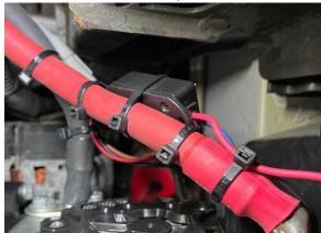
6.5. Run the regulator harness up to the regulator and secure it adequately using zip ties as pictured below:
