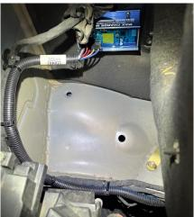
6.6. Connect regulator harness to regulator. The single red wire goes to pin 9. The temperature sensor ground goes to pin 5 and the sensor positive goes to pin 6. See picture below:
