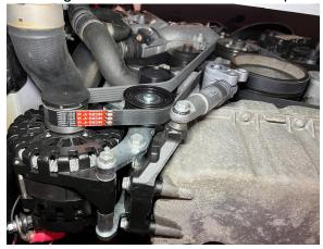
5.3. Install regulator onto regulator bracket using supplied 10-32 screws and nuts, and then bolt the regulator/bracket assembly onto the studs on the passenger side of the HVAC air intake as pictured below:
