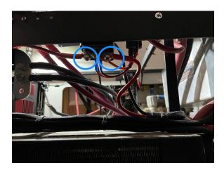
1.12. Remove all wires from the Victron BP65 (blue box) if still installed. It will be necessary to remove the ground wire for the relay from the negative bus bar
