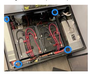
1.4. Remove seven screws holding front wooden panel on
