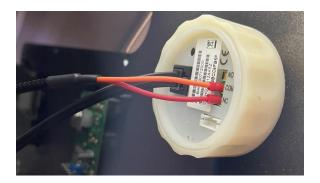
2.3. Remove the black connector from the back of the House Battery switch and replace it with the black connector with the ORANGE and GREEN wires
