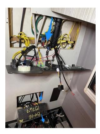
This should end up where the main harness, solar wires and DC panel wires come off of frame 1.9.1. (bottom corner of battery tray)
