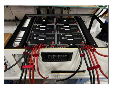
With both the negative (black) and positive (red) cables disconnected, drape the cable assemblies over the front of the bench seat as shown.
