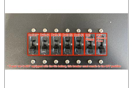
Shut off all the breakers on the RoamRig system. The breakers are located in the battery compartment on the driver's side rear compartment of the van.
