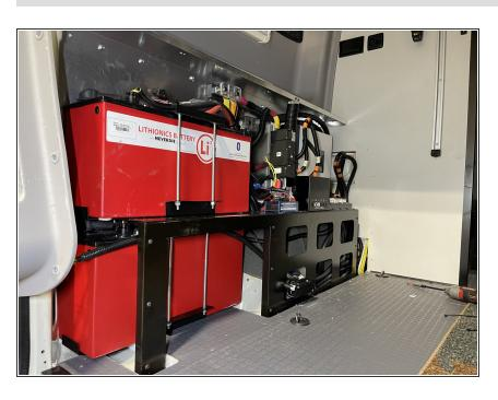
With the batteries installed, ensure all the connections are secure, the plastic bus bar covers are in place, and all wires are properly secured/routed.
