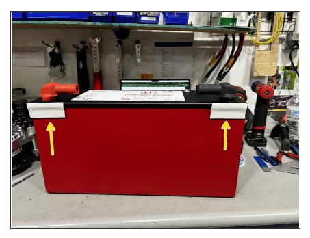
Before installing the battery, install the provided foam tape strips to the battery as shown in the first image.
