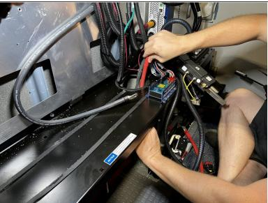
Route the 2nd battery cables up through the hole in the shelf. Ensure the CAN connector harness
