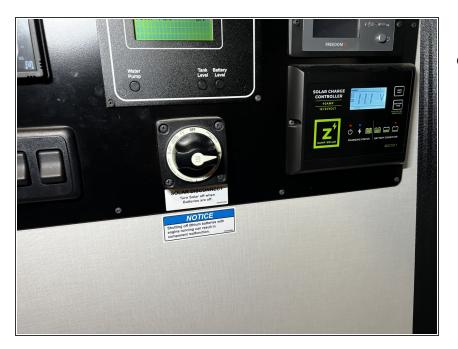
Turn the solar disconnect knob to the ON position on the control panel in the van.
