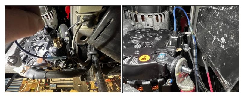
Insert the field wire connector into the alternator. Ensure the connector is fully seated into the alternator.
