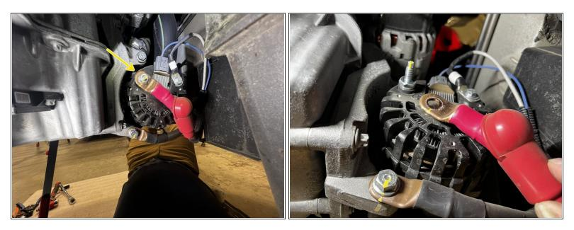
• Using a 13mm socket and wrench remove the positive cable from the back of the alternator.
