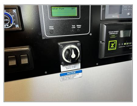
• Turn the solar disconnect knob to the "OFF" position on the control panel in the van.
